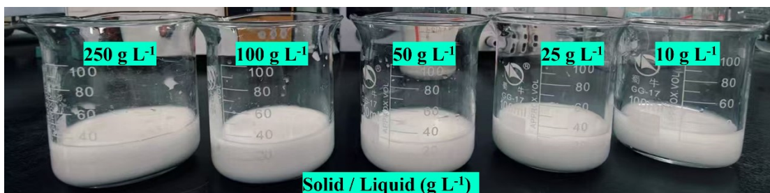
Fig. S6. Digital photographs of leaching slurries under different solid-to-liquid ratios (10-250 g·L -1 )
