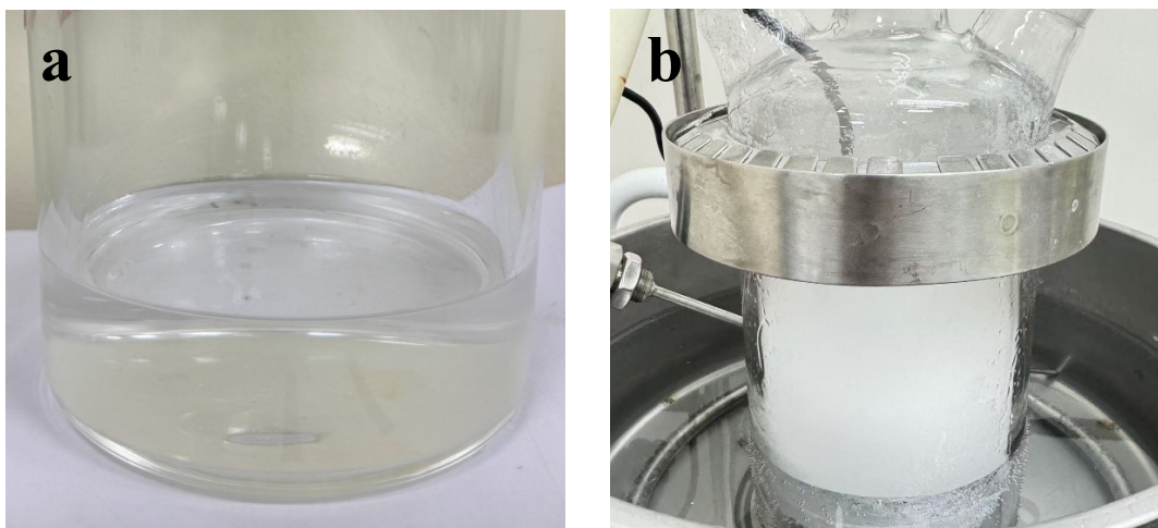
Fig. S1 (a) Liquid mixtures used for microdroplets reaction and (b) Ultrasonic atomization device for synthesizing dimethyl phthalate microdroplets.
