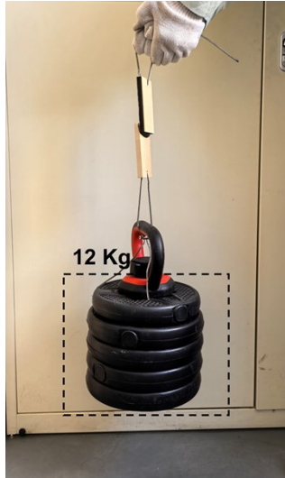
Figure S12. Image of LPT adhesives-bonded wood sheets to support a dumbbell weighing 12 kg (185 cm of height) with a bonding area of 18.5 x 48.5 mm 2 .
