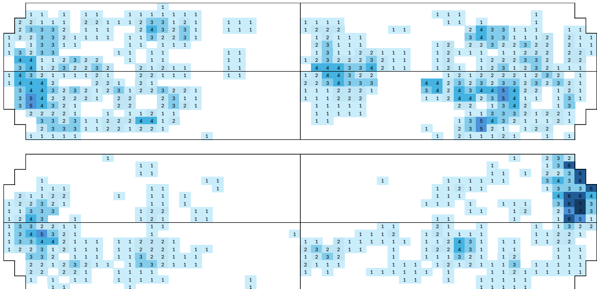
Figure S 23 Hit maps of the h10-d15 Cylinder at a frequency of 25 Hz. Top: Front view; Bottom: Bottom view. The hit counts were prepared by analyzing 6 videos of 0.5 s exposure. All hit numbers correspond to an assigned color.
