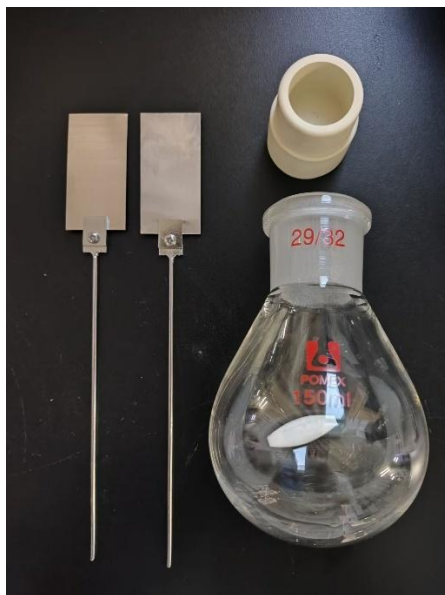
Figure S2. Electrolysis set-up for gram-scale experiment.
