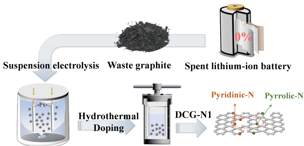
Figure S2. Schematic illustration of the preparation of defect-controllable N-doped graphene (DCG-N1) from SG via the RDWC-based exfoliation-doping route.
