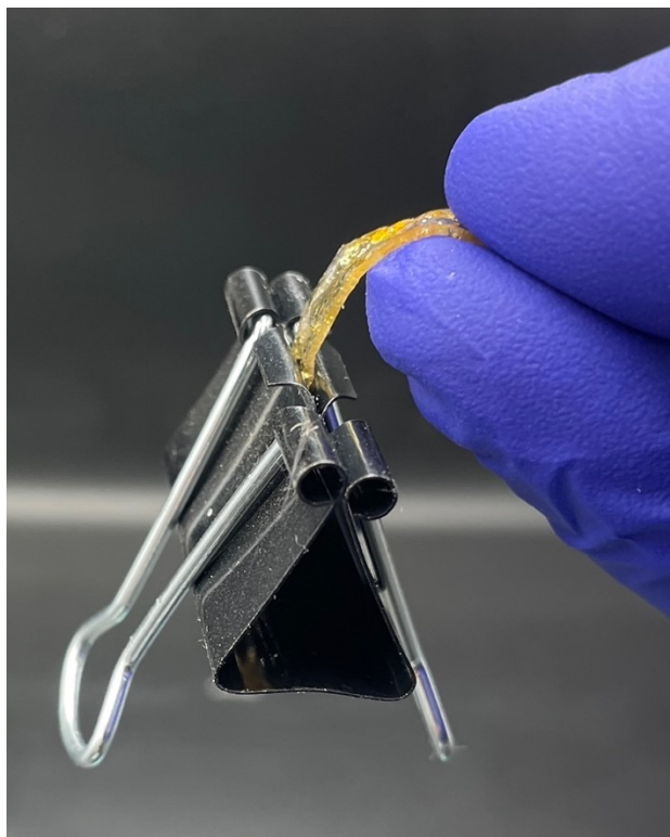
Figure S2. Photo of the sample produced with non-reactive tertiary amine catalyst, Dimethylethanolamine (DMAE) at 23 °C.
