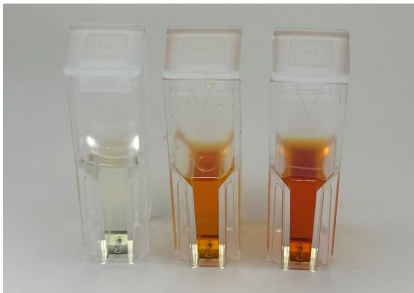
Figure S7. Photographs of control HK/G6PDH assay (left), 20-fold diluted starch hydrolysate obtained at pH 5.2 after 1 hour at room temperature (center), and 20-fold diluted starch hydrolysate obtained at pH 5.2 after 1 hour at 60 °C (right).
