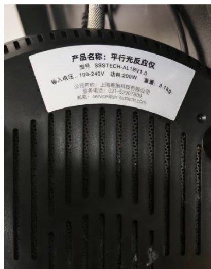
Figure S14. Photoreactor used in this study. A) Photoreactor. B) Manufacturer information: Shanshi Technology Co., Ltd. (Shanghai, China); model: SSSTECH-AL1BV1.0.
