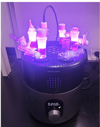
Figure S14. Photoreactor used in this study. A) Photoreactor. B) Manufacturer information: Shanshi Technology Co., Ltd. (Shanghai, China); model: SSSTECH-AL1BV1.0.
