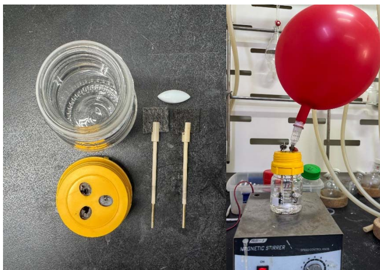
Figure S2. Electrolysis setup for the gram scale experiment.
