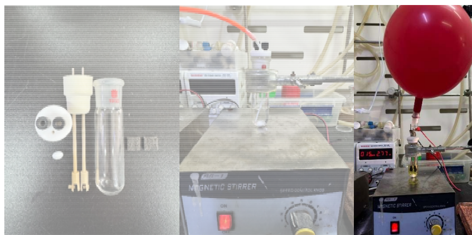
Figure S1. Electrolysis setup for the standard reaction experiment
