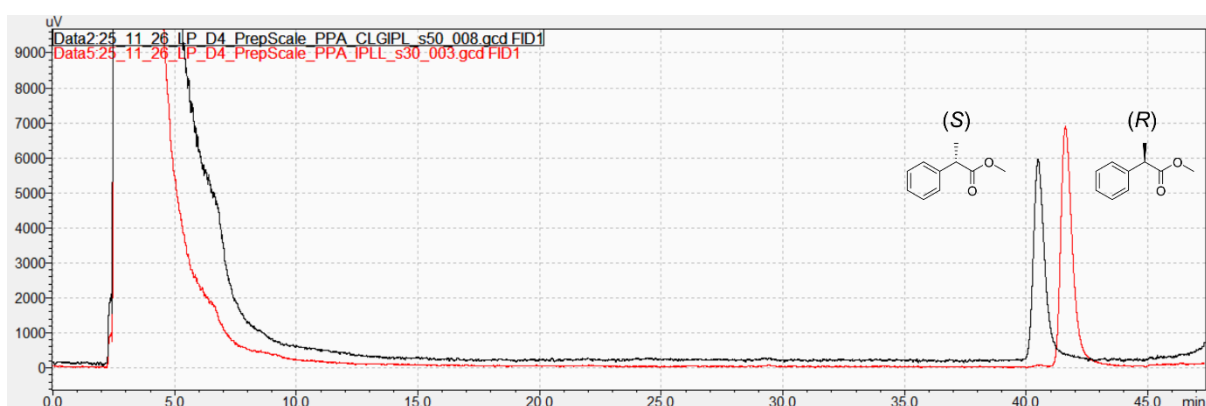
Figure S14. Exemplary GC-FID chromatogram of the converted 2-methyl-2-phenylmalonate with (S)-selective AMDase ICPLLG (black) superimposed with (R)-selective AMDase IPL (red). The samples were derivatized with TMS-CH 2 -N 2 according to Section 2.2 . Retention times: methyl (S)-2-phenylpropanoate = 40.5 min, methyl (R)-2-phenylpropanoate = 41.6 min.
