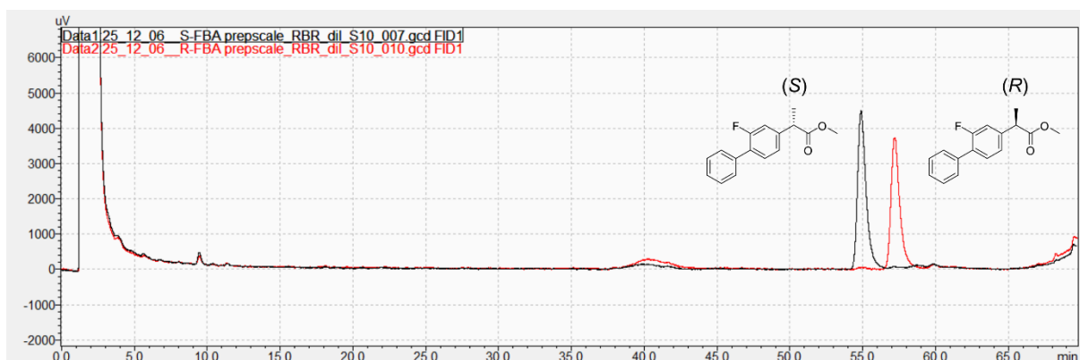
Figure S13. Exemplary GC-FID chromatogram of the converted flurbiprofen malonate with (S)-selective AMDase ICPLLG (black) superimposed with (R)-selective AMDase IPL (red). The samples were derivatized with TMS-CH 2 -N 2 according to Section 2.2 . Retention times: (S)-flurbiprofen-methylester = 55.0 min, (R)-flurbiprofen-methylester = 57.4 min.
