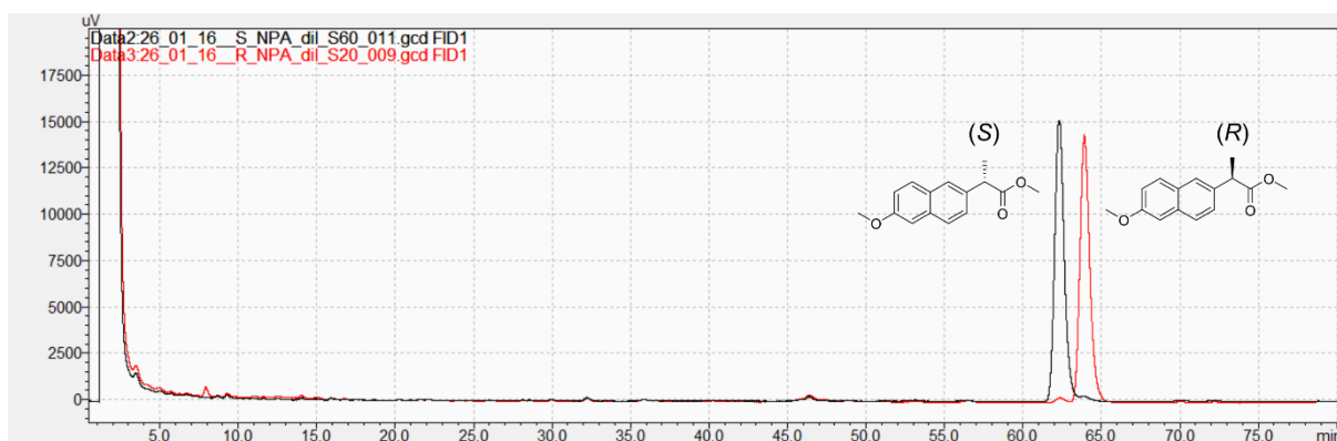
Figure S12. Exemplary GC-FID chromatogram of the converted naproxen malonate with (S)-selective AMDase ICPLLG (black) superimposed with (R)-selective AMDase IPL (red). The samples were derivatized with TMS-CH 2 -N 2 according to Section 2.2 . Retention times: (S)-Naproxen-methylester = 62.4 min, (R)-Naproxen-methylester = 64.0 min.
