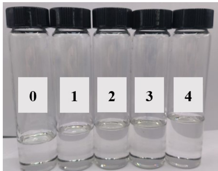
Figure S2 Digital images of DES with varying water content ( \text{ChCl}:\text{CA}:\text{H}_2\text{O}=1:1:\text{X} , \text{X}=0-4 ).
