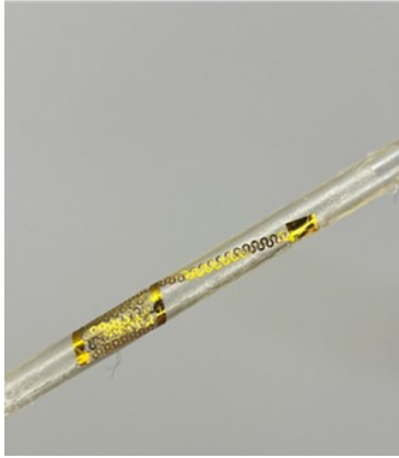
Figure S11 Integration of the serpentine electrodes to a tubular-shaped platform with various diameters, starting from 2 mm to 5 mm. The 2.8 mm is selected as the benchmark diameter because it is the typical dimension of the EVD catheter, the basis of our current design.
