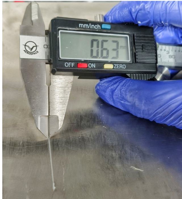
Fig. S1 Digital image illustrating the measurement of line width using a vernier calliper and the corresponding width achieved during NFEP at optimized parameters determined through Taguchi experiments.
