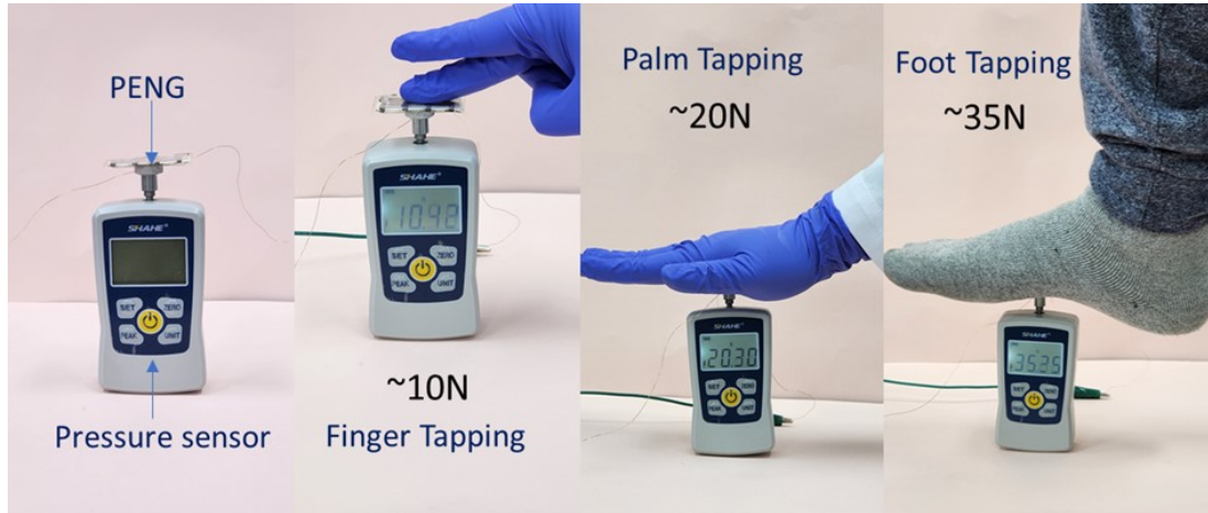
Figure S11. Digital images illustrating the measurement of applied forces using a pressure sensor during different actuation modes.
