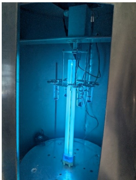
Figure S 7: Image of the custom-made photo-reactor equipped with a 365 nm UV-lamp.
