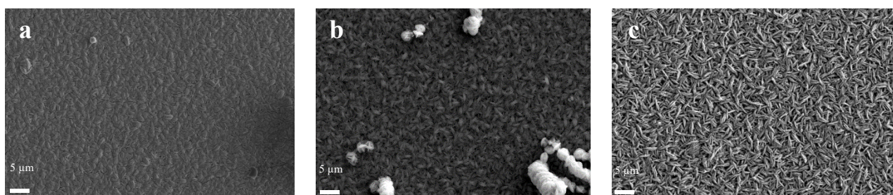
Figure S5: SEM images of as-prepared \text{CuFeO}_2 thin films derived from powders synthesized at (a) 110 °C, (b) 140 °C, and (c) 170 °C. Films from higher temperature syntheses show denser packing and improved continuity.
