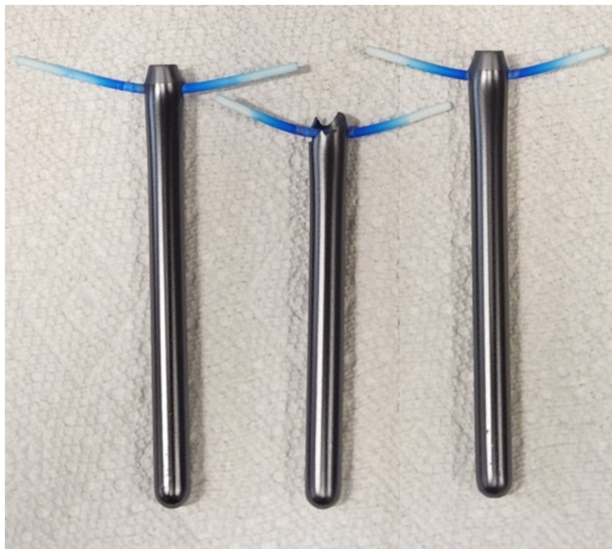
Figure S1: Sintered NiO-BCZYYb7111//BCZYYb7111 with the hanging alumina rods.
