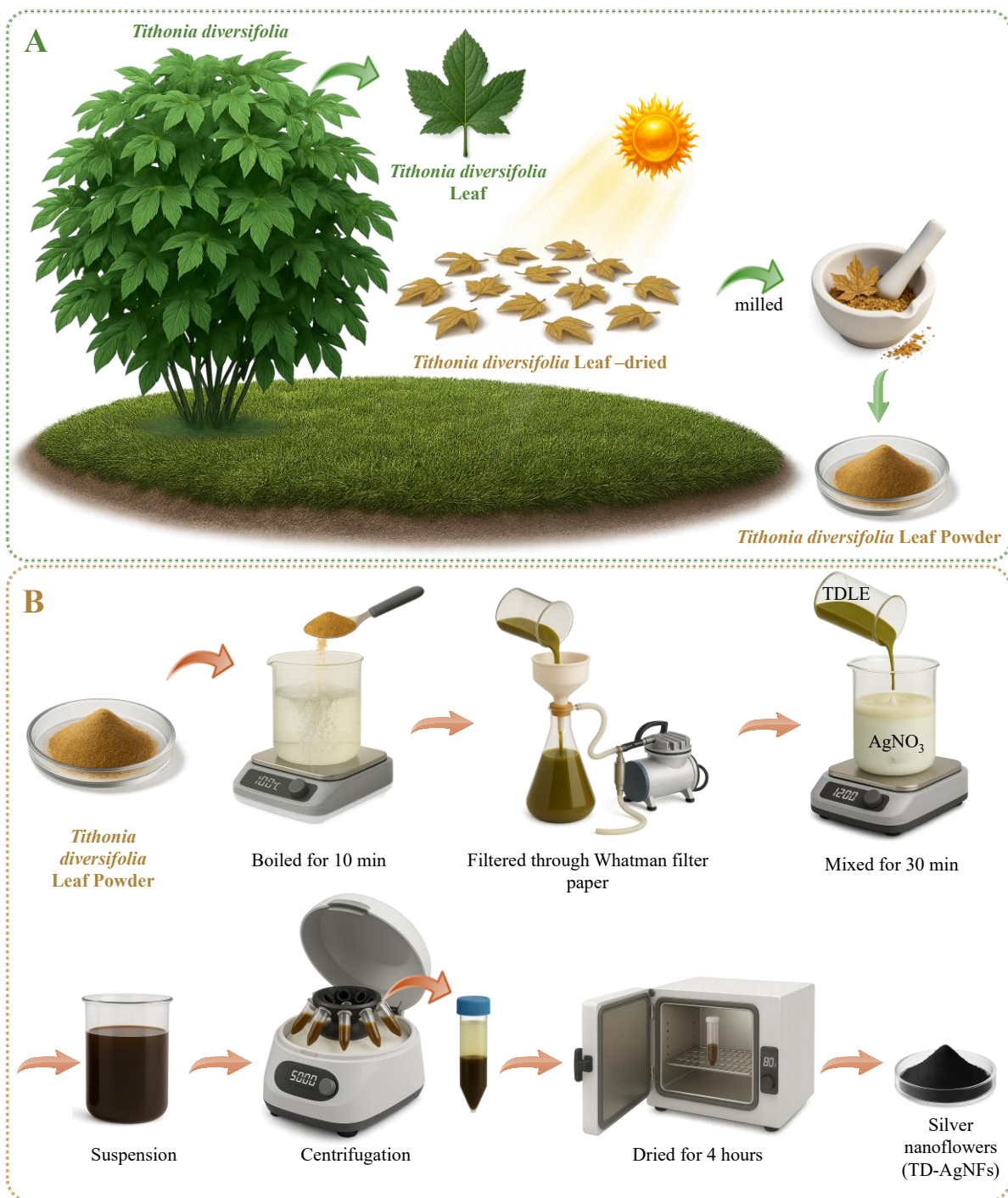
Supporting Fig. 1. Green synthesis of silver nanoflowers (AgNFs) using Tithonia diversifolia leaf extract (TDLE). (A) Preparation of plant precursor: T. diversifolia leaves were sun-dried and milled to a fine powder. (B) Synthesis scheme: the leaf powder was boiled in water for 10 min and filtered through Whatman paper to obtain TDLE; the extract was mixed with aqueous AgNO 3 for 30 min to reduce Ag + , producing a brown suspension; the product was collected by centrifugation and washing, then dried at 60 °C for 4 h to yield TD-AgNFs.
