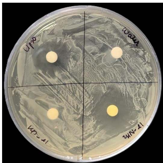
Fig. S10. Zone of inhibition test using sterile discs.
