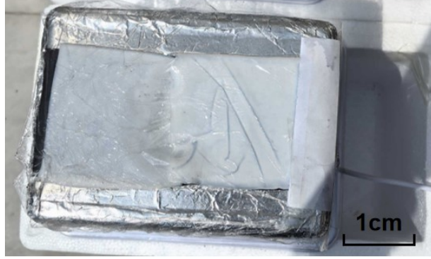
Figure S20. The turbid NA-Li window under the natural sun irradiation for greenhouse experiment.
