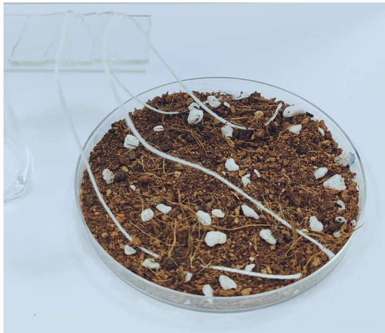
Figure S13. The water collection and transport pictures of NA-Li by sewing the cotton thread in the NA-Li hydrogel.
