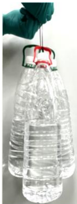
Figure S27 TPU-Q 75 U 25 specimen loaded weight of 2.5 kg after self- self-healing under NIR irradiation at I_{808} of 200 \text{ mW}\cdot\text{cm}^{-2} within 10 min.
