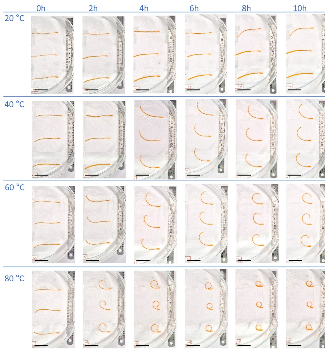
Figure S8. Temperature- and time-dependent actuation behavior of the printed specimen. Photographs of the specimen immersed in water at 20, 40, 60, and 80°C (rows) captured at 0, 2, 4, 6, 8, and 10 hours (columns). Scale bar: 30 mm.
