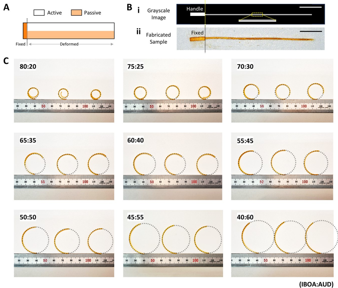
Figure S6 g-DLP printing of bilayer specimens and characterization. A Design of a bilayer specimen. B (i) Grayscale image used for g-DLP fabrication and (ii) the fabricated specimen. Each scale bar corresponds to 10 mm. C Deformed shapes of g-DLP-printed specimens after thermal activation for nine different IBOA:AUD compositions. Dashed circles are fitted circles used to calculate curvature.
