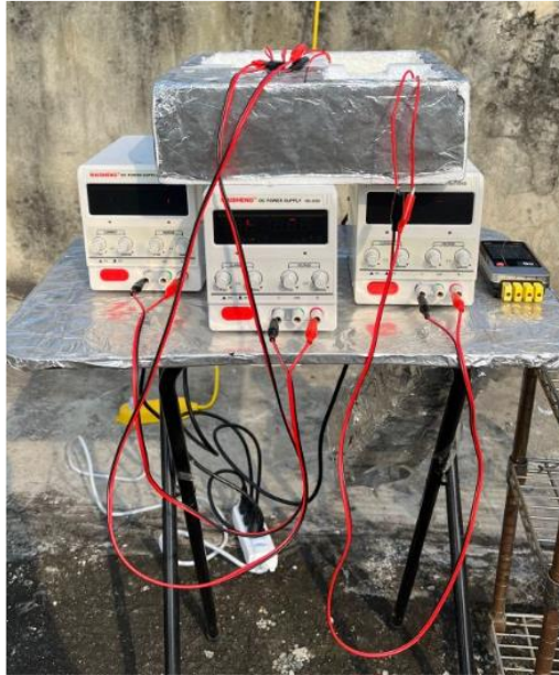
Fig S49. Photograph of an outdoor cooling test placed horizontally with a heat load of 600 \text{ W/m}^2 .
