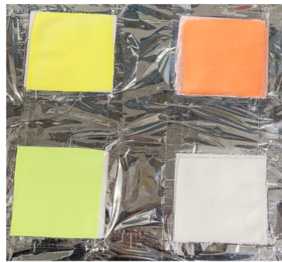
Fig S23. Outdoor test photos of TBC when placed horizontally at room temperature. Ambient temperatures were tested using a Stevenson screen.
