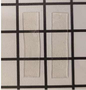
Figure S21. Photograph of SrGelCas (left) and ZnGelCas (right) organohydrogel strips demonstrating their high optical transparency.
