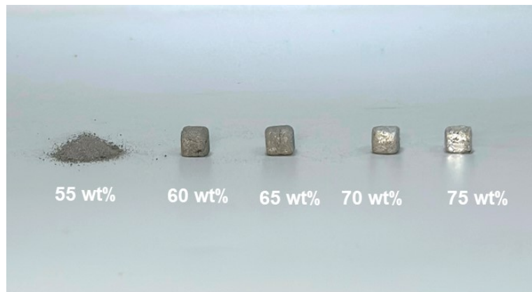
Figure S7. Optical images of sample morphologies at different LM contents (wt%). From left to right, the LM contents are 55 wt%, 60 wt%, 65 wt%, 70 wt%, and 75 wt% in sequence.
