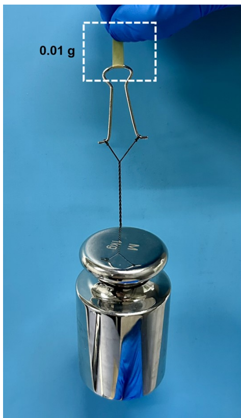
Fig. S11. Optical image showing ANF-5000 supporting a load of 1 kg.
