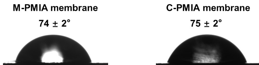
Fig. S8 Images of water contact angles of the M-PMIA and C-PMIA membranes.
