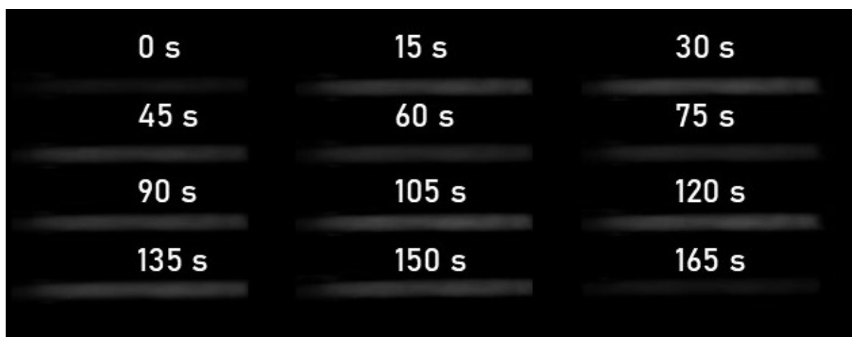
Figure S29. The intensity maps recorded in the G channel obtained from photos of the luminescence of the strip of \text{LiYO}_2:0.1\%\text{Tb}^{3+} phosphor deposited on the metal nozzle of the heat gun captured as a function of time.
