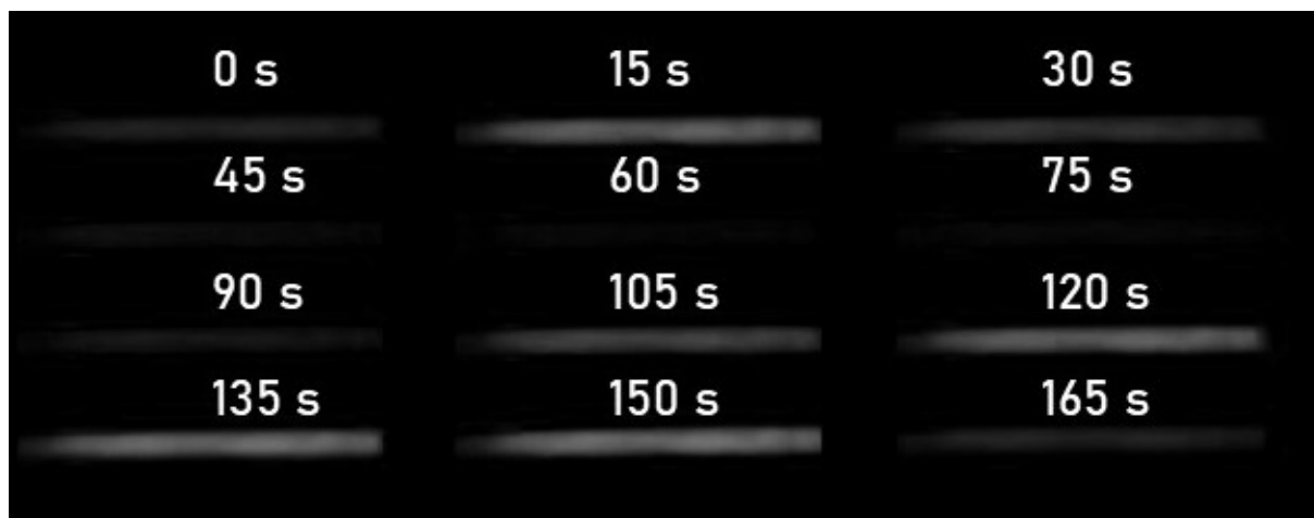
Figure S28. The intensity maps recorded in the B channel obtained from photos of the luminescence of the strip of \text{LiYO}_2:0.1\%\text{Tb}^{3+} phosphor deposited on the metal nozzle of the heat gun captured as a function of time.
