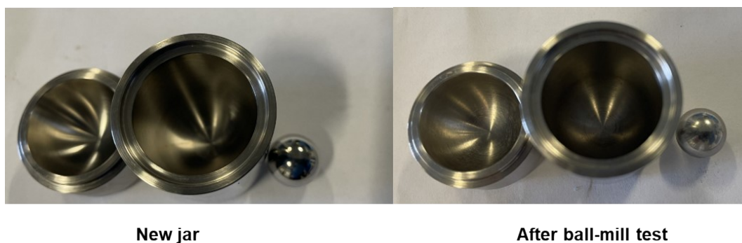
Figure S14 | Image of new ball milling jar and after milling with starting materials at 23.3 Hz for 50 minutes
