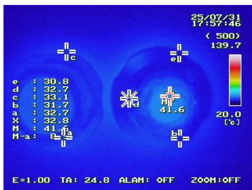
Figure S6. Thermographically derived temperature (41.6 °C) inside the milling jar after grinding for 60 min at 30 Hz.
