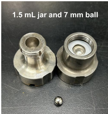
Figure S2. Stainless jar (1.5 mL) and balls (7 mm) used in this study.
