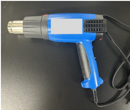
Figure S3. The temperature-controllable heat gun Takagi HG-1450B used in this study.
