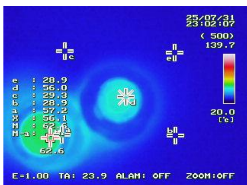
Figure S7. Thermographically derived temperature (62.6 °C) inside the milling jar after grinding for 60 min at 30 Hz.
