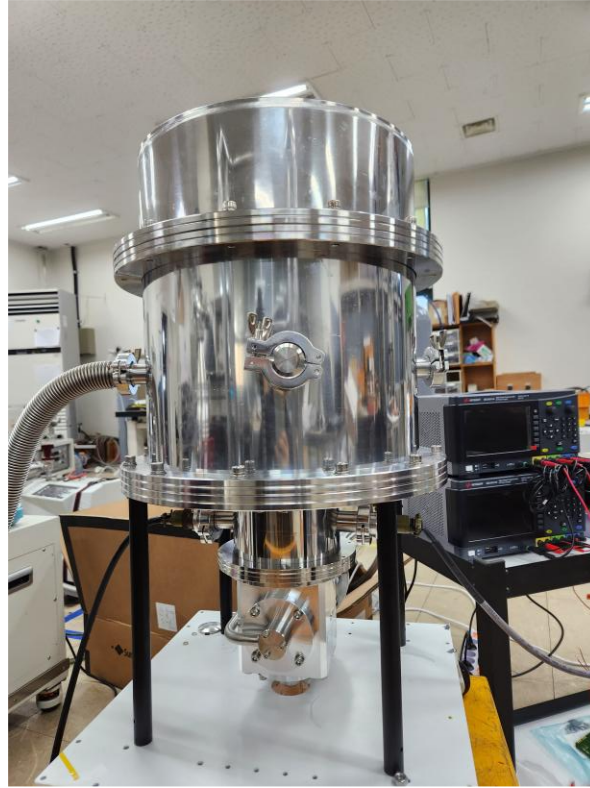
Figure S1. Photograph of the low-temperature electrical measurement setup. The device was mounted inside a cryostat and cooled using a Gifford–McMahon (GM) cryocooler, enabling stable temperature control over the range investigated in this study. Gate and drain voltages were applied, and the drain current was measured using a source-measure unit.
