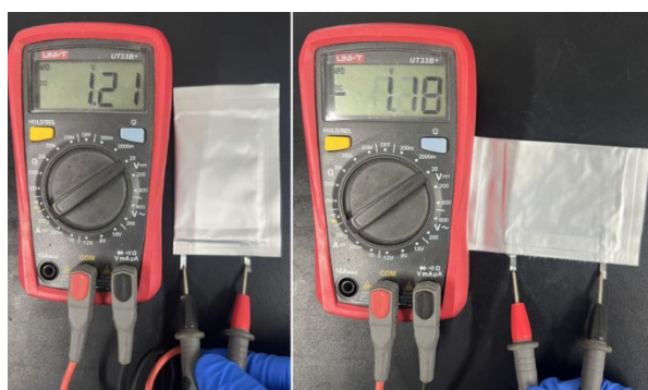
Figure S10. Open-circuit voltage of one pouch cell.
