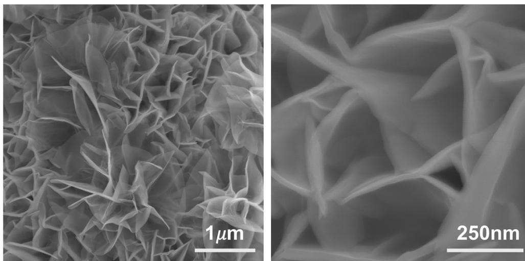
**Figure S3.** SEM images of  $\alpha$ - $\text{MnO}_2$  nanosheet obtained.
