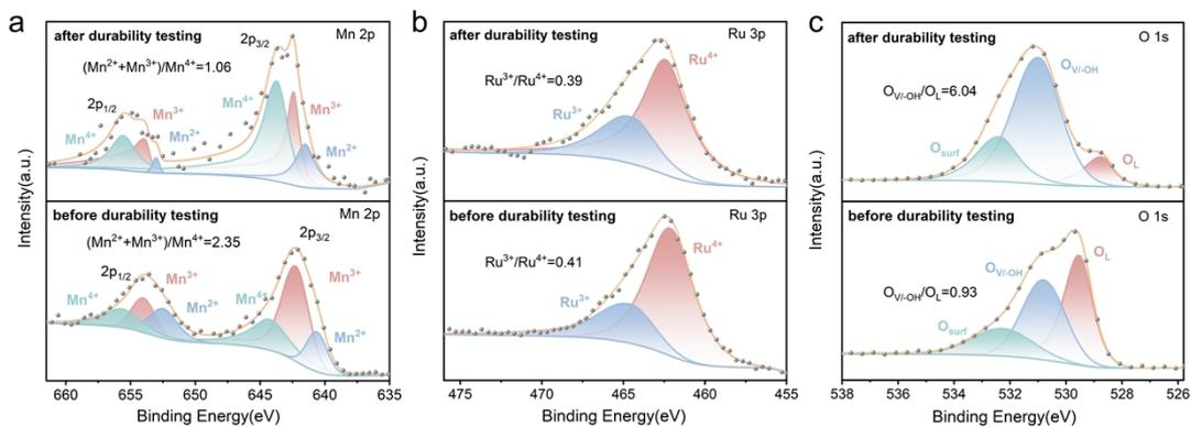
**Figure S25.** High-resolution XPS spectra of Ru-MnO<sub>2</sub> NW after cv: (a) Mn 2p, (b) Ru 3p and (c) O 1s.
