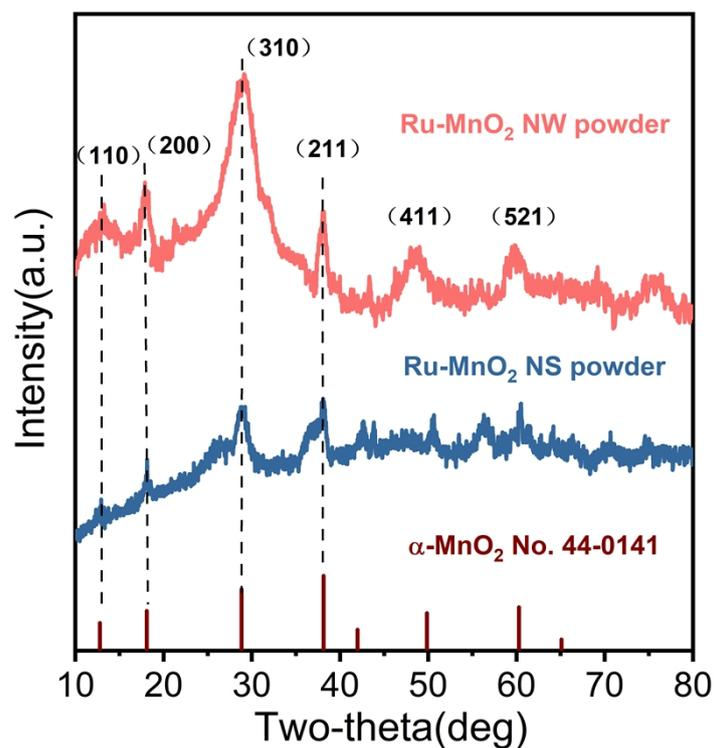
**Figure S10.** XRD patterns of carbon cloth, Ru-MnO<sub>2</sub> NW powder and Ru-MnO<sub>2</sub> NS powder.
