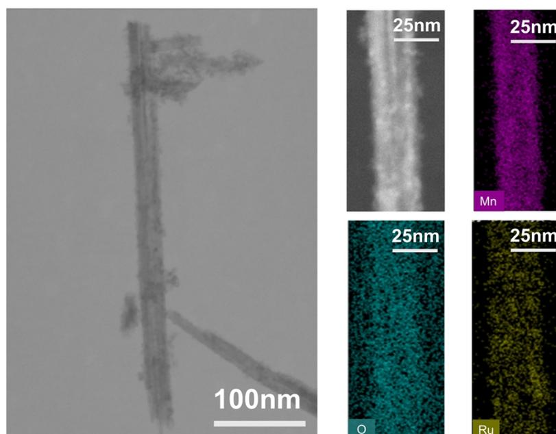
**Figure S23.** TEM image of Ru-MnO<sub>2</sub> NW after cv and EDS elemental maps of Ru-MnO<sub>2</sub> NW after cv (Mn, O and Ru).
