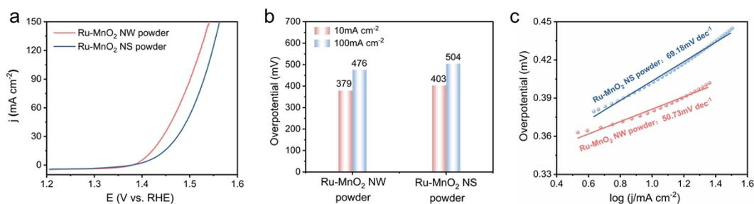
**Figure S16.** (a) LSV curves of Ru–MnO<sub>2</sub> NW powder and Ru–MnO<sub>2</sub> NS powder in 0.5 M H<sub>2</sub>SO<sub>4</sub>, (b) Comparison of overpotentials required to reach current densities of 10 and 100 mA cm<sup>-2</sup>, (c) Corresponding Tafel plots derived from the polarization curves.
