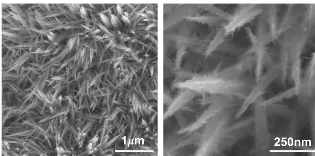
**Figure S2.** SEM images of  $\alpha$ -MnO<sub>2</sub> nanoneedles obtained.
