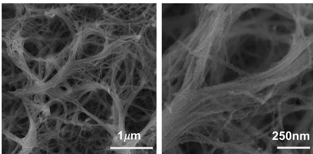
**Figure S22.** SEM images of Ru-MnO<sub>2</sub> NW after cv.
