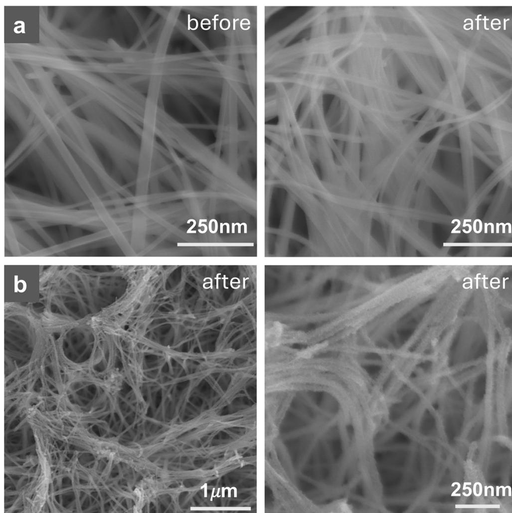
**Figure S4.** SEM images: (a)  $\text{MnO}_2$  NW before and after Ru ion exchange; (b) Ru- $\text{MnO}_2$  NW with different sizes after calcination at 200 °C.
