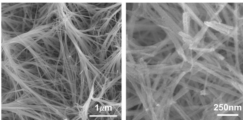
**Figure S1.** SEM images of  $\alpha$ -MnO<sub>2</sub> nanowires obtained.
