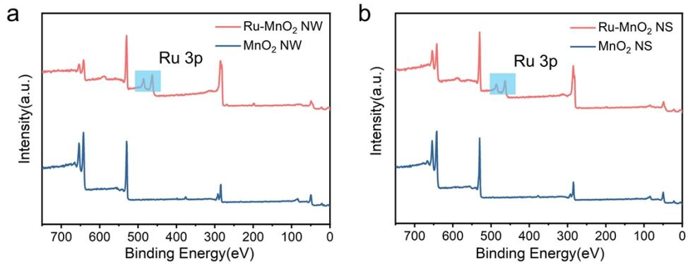
**Figure S13.** High-resolution XPS full spectrum of (a) Ru-MnO<sub>2</sub> NW and MnO<sub>2</sub> NW, (b) Ru-MnO<sub>2</sub> NS and MnO<sub>2</sub> NS.
