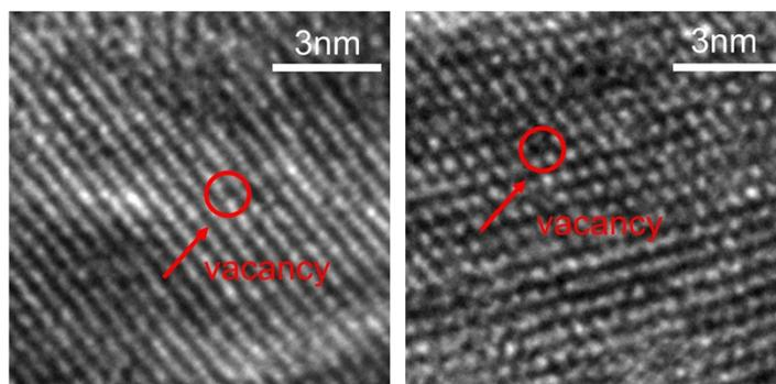
**Figure S7.** Vacancy defects of Ru-MnO<sub>2</sub> NW observed via TEM.
