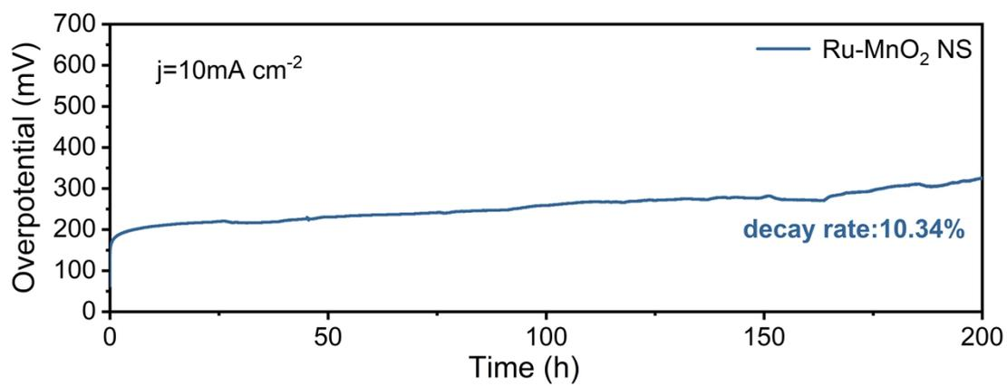
**Figure S21.** Long-term chrono potentiometric stability test of Ru-MnO<sub>2</sub> NS at a constant current density of  $10 \text{ mA cm}^{-2}$ .
