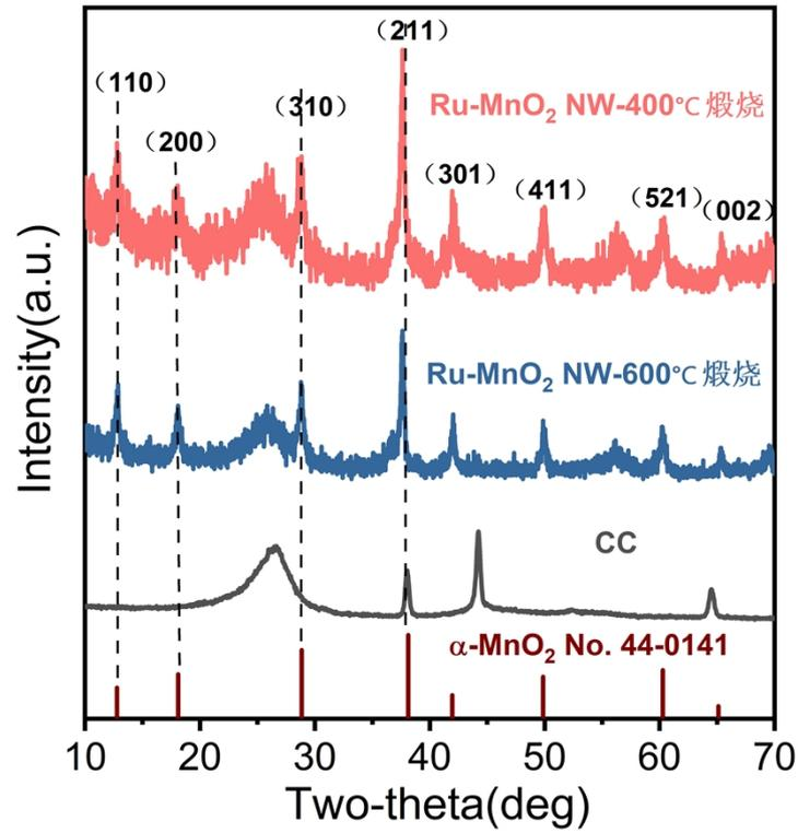
**Figure S12.** XRD patterns of carbon cloth and Ru-MnO<sub>2</sub> NW calcined at 400 °C and 600 °C.
