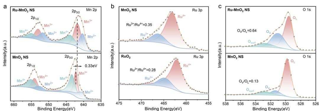
**Figure S14.** High-resolution XPS spectra of Ru–MnO<sub>2</sub> NS: (a) Mn 2p, (b) Ru 3p and (c) O 1s, evidencing a reduced Mn redox state, an increased vacancy-associated oxygen component, and a higher Ru<sup>3+</sup>/Ru<sup>4+</sup> fraction relative to RuO<sub>2</sub>.
