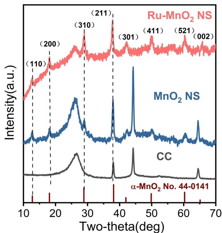
**Figure S11.** XRD patterns of carbon cloth, MnO<sub>2</sub> NS and Ru-MnO<sub>2</sub> NS, showing retention of the  $\alpha$ -MnO<sub>2</sub> phase without detectable crystalline RuO<sub>x</sub>.
