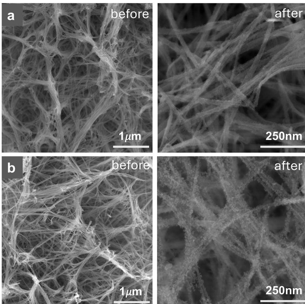
**Figure S5.** SEM images of Ru-MnO<sub>2</sub> NW before and after calcination at different temperatures: (a) 400 °C, (b) 600 °C.
