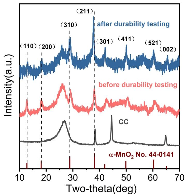
**Figure S24.** XRD patterns of carbon cloth, Ru-MnO<sub>2</sub> NW and Ru-MnO<sub>2</sub> NW after cv.
