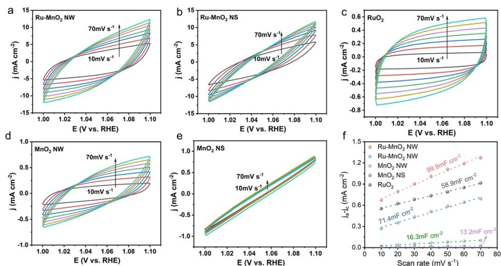
**Figure S18.** Electrochemical cyclic voltammetry scans recorded for (a) Ru–MnO<sub>2</sub> NW, (b) Ru–MnO<sub>2</sub> NS, (c) commercial RuO<sub>2</sub>. (d) MnO<sub>2</sub> NW, (e) MnO<sub>2</sub> NS, (f) Linear fitting of the capacitive currents versus cyclic voltammetry scans for these catalysts.
