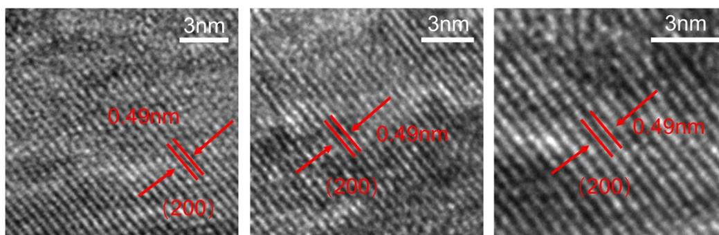
**Figure S6.** TEM lattice fringes of Ru-MnO<sub>2</sub> NW.
