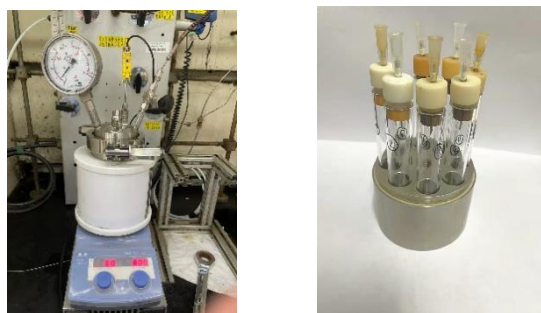
Figure S1. High-pressure steel autoclave and parallel reaction modulator.
