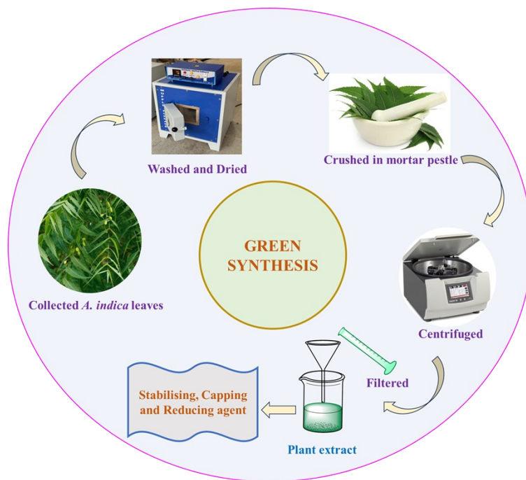
Figure 3s. Preparation of leaf extract and its role in nanoparticle synthesis
