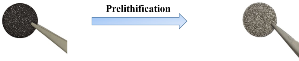
Figure S10 Optical photographs of the CuO-Ag@NF material before and after prelithiation.
