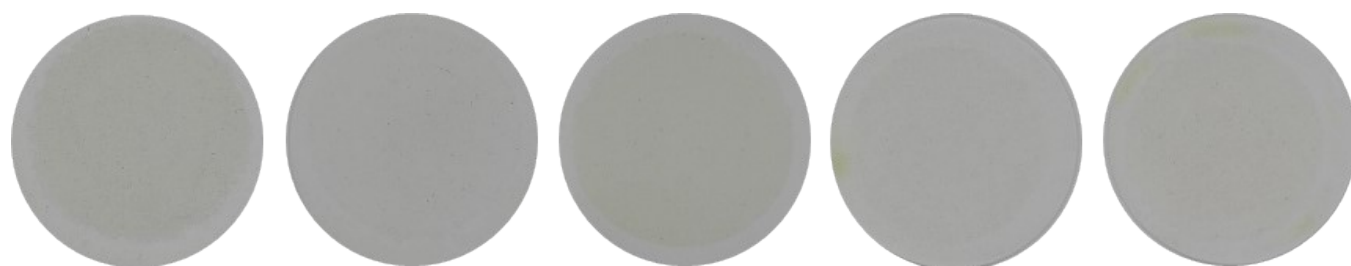
Figure S3. Photographs of the filter membranes after filtration of the binary-solute 0.08 M \text{CuCl}_2 -0.16 M \text{NaH}_2\text{PO}_2 -Ethaline system reacted at different temperatures (353–393 K) for 6 h.
