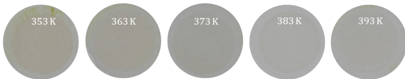
Figure S2. Photographs of the filter membranes after filtration of the single-solute 0.08 M \text{CuCl}_2 -Ethaline system reacted at different temperatures (353–393 K) for 6 h.
