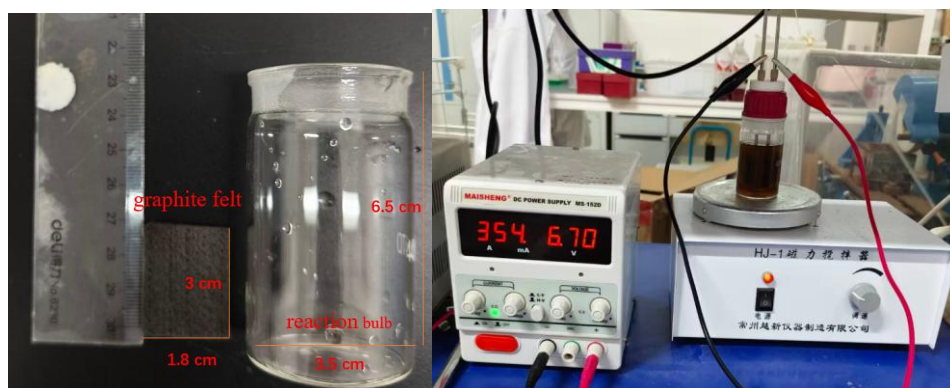
Figure S3. Electrolysis setup
