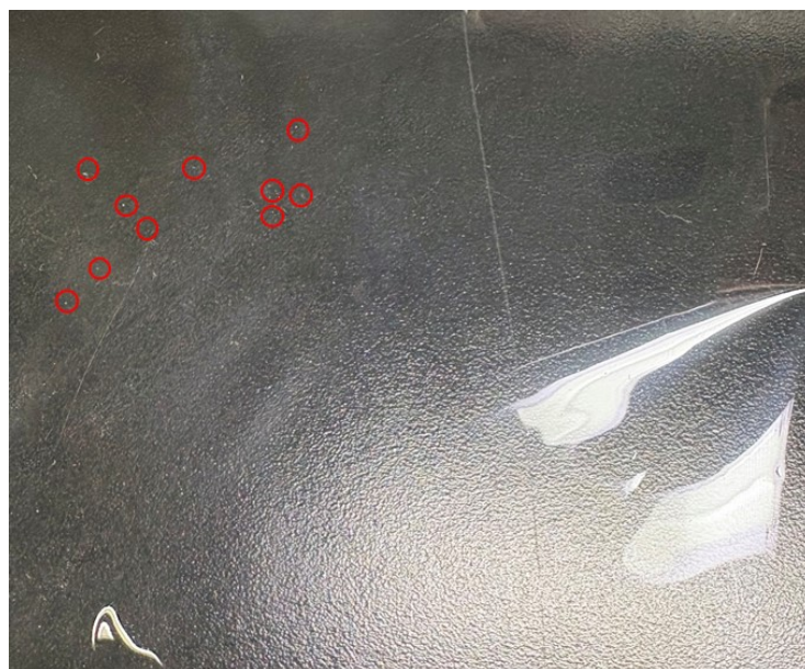
Fig. S6 Surface defects (pinholes and agglomerates) observed on the CeO 2 NPs reinforcing filler/PET film.
