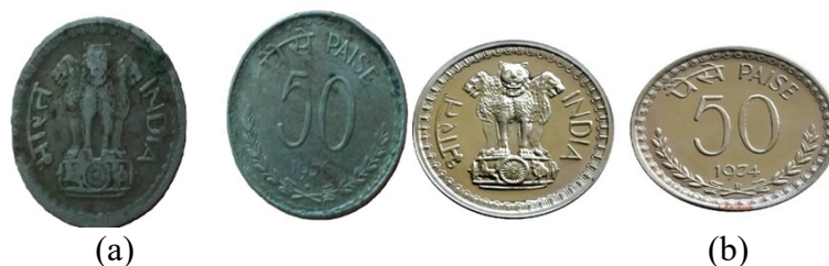
Figure S4 Fifty paise coin used as working electrode.
