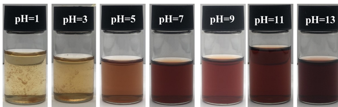
Figure S1. Dispersion stability of BWTNPs solution under different pH conditions (mass concentration of 0.08 wt%).
