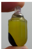
Figure S14: Tubes of the dispersion in EMIM TFSI after 42 h of ultracentrifugation at 50000 rpm.
