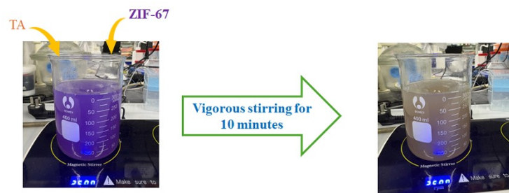
Scheme S1. Digitally captured images showing the chemical etching procedure for ZIF-67 MOF modification.
