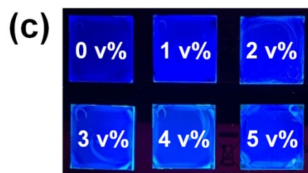
Fig. S2 Photoluminescence images of perovskite films prepared with iron additive concentrations (0–5 v%) under UV lamp illumination. (a) Red films. (b) Green films. (c) Blue films.
