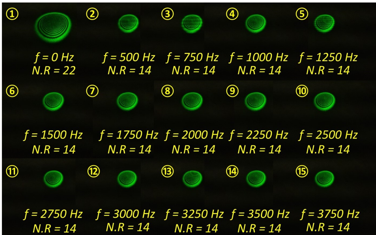
Figure S9. Mechanical chopper operating at high Frequency for 532 nm. (0-3.75 kHz).
