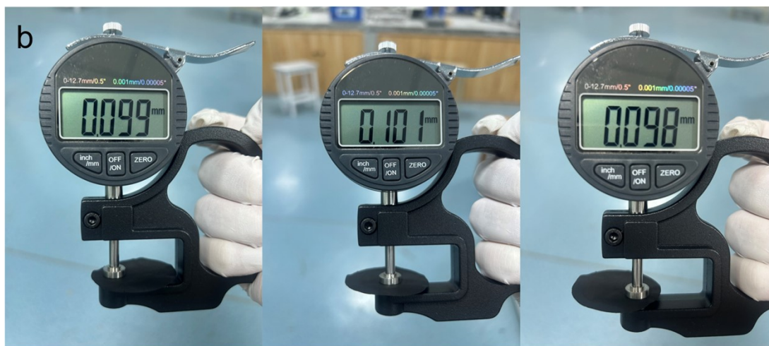
Fig. S2. (a) Schematic illustration of the fabrication of flexible and freestanding P-V_2O_3@C film electrode. (b) The thickness of the electrode was measured at different positions using a thickness gauge.
