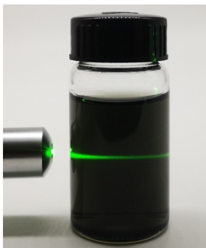
Fig. S2 The Tyndall phenomenon of the as-obtained \text{Ti}_3\text{C}_2\text{T}_x MXene solution
