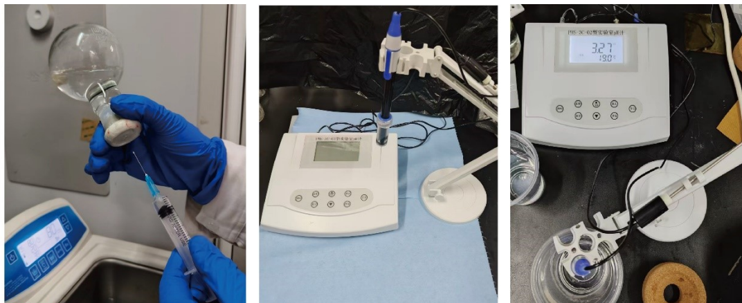
Figure S11. The pH of the liquid was measured after 2 h of ultrasonic contact catalysis.
