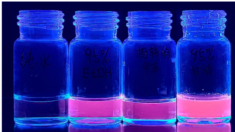
Figure S8. UV-vis absorption spectra and photograph of the Au 22 SG 18 nanocluster in various solvents (left to right: water, 95% EtOH, toluene and 95% Glycerol).
