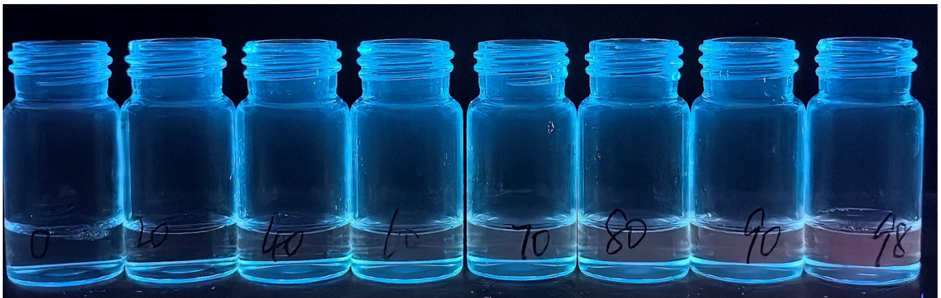
Figure S11. photograph of the \text{Au}_{21}\text{Cys}_{17} nanocluster in glycerol/water solutions of varying concentrations (lables on the vases is the volume ratio of glycerol).
